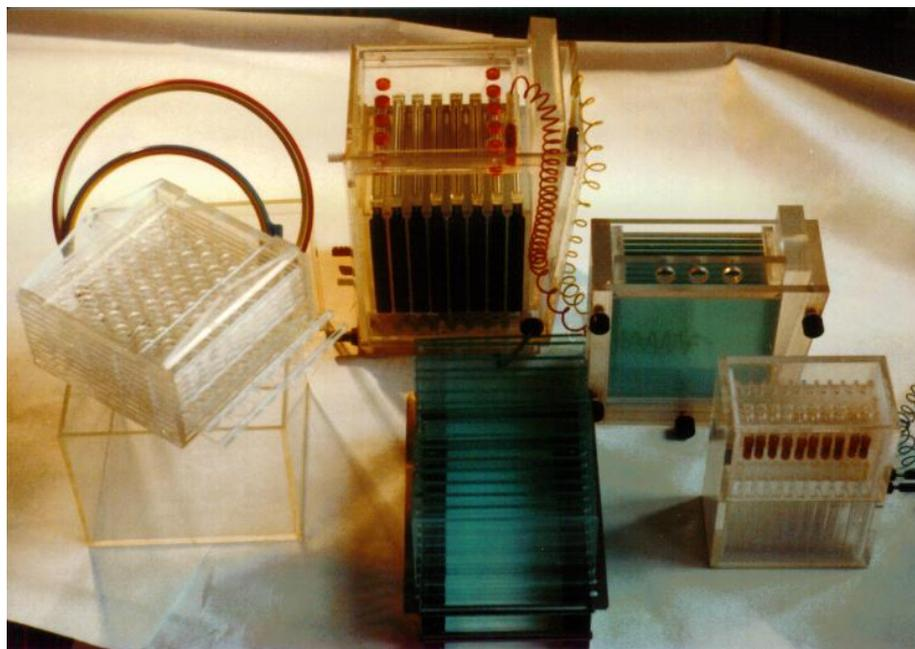
The set of tools was specially developed for proteomic researchers. It is intended for comparative analysis of complicated protein mixtures using synchronous two-dimensional gel electrophoresis in eight slabs of polyacrylamide gel. The design provides excellent reproducible separation of proteins. It greatly improves throughput and is easy in operation.
