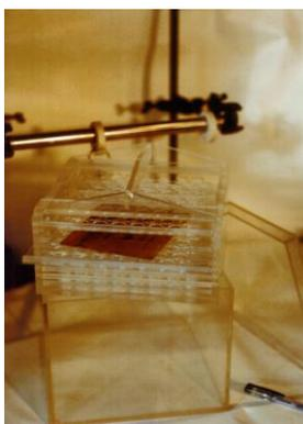
The device is a plexiglass cell with a cover. Rectangular basket carrying 8 removable perforated shelves is put inside the cell. Extracted from cassettes after electrophoresis gel slabs are placed on the basket shelves. Then the basket is put into the cell containing washing or developing solutions. The shaking of solution is carried out by slow basket swing due to its connection with rotating eccentric shaft outside. The device saves time and guarantees stability of the results.
